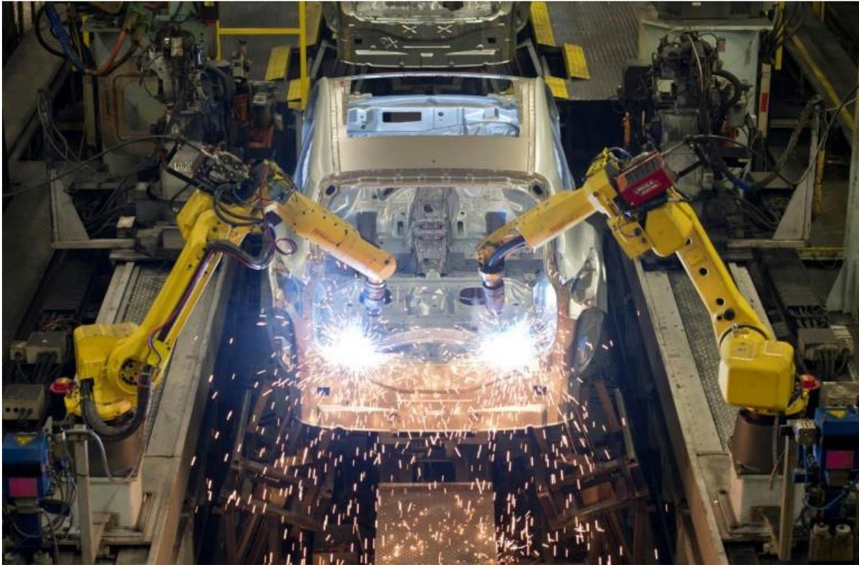
*Automation has transformed the productivity of manufacturing since industrial robots first started painting, cutting, welding and assembling in the 1960s. (Photo: AFP)*
